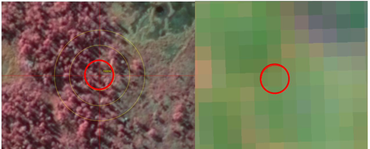
Figure 2.8 – Color-IR Orthophoto (left), SPOT satellite image (right, with NIR, SWIR and Red as RGB display) over a mountain birch forest, where darkening effect of tree shadows can be seen in both images. For orientation, the red circle is the same plot in both images.
