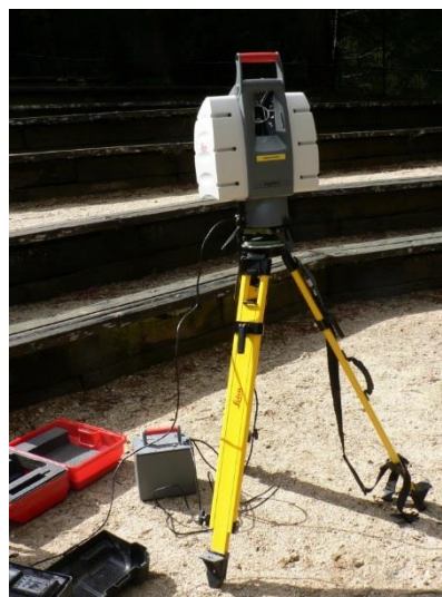
Figur 6.18 The Leica terrestrial laser scanner can be used to scan buildings, rock formations, forests, etc., to produce a 3D model consisting of
