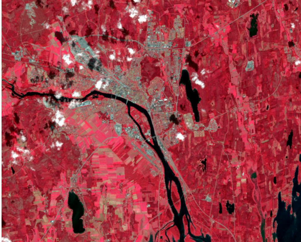
Figure 4.2 – Subset of a Landsat-8 image 2014/08/13 over Umeå shown as NIR (band 5), Red (band 4), Green (band 3) in RGB display.
