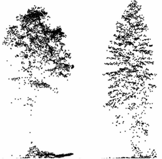
Figur 6.15. Point clouds profiles from pine and spruce, the pulse density of about 50 m -2 . Image: Johan Holmgren, SLU.
