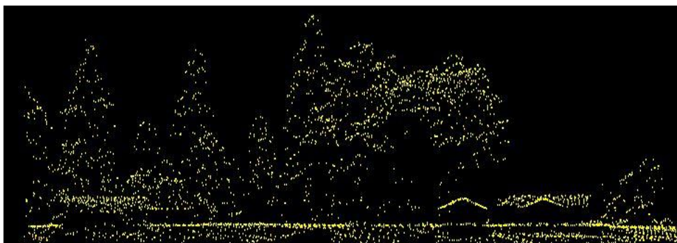
Figur 6.8. Profile of laser point cloud where trees and buildings are clearly visible. The image is based on data from the National Land Survey. © Lantmäteriet, i2012/107.
