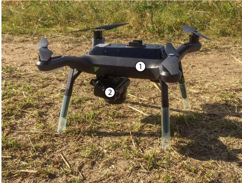
Figure 3.2 Quadcopter (1) of 3D Robotics model Solo. On this platform, there is a Sony Alpha SLR 5100 camera (2) with a 20mm lens.
