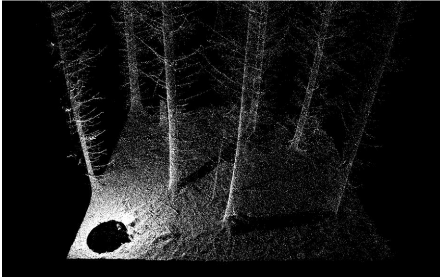
Figur 6.19 Examples of a TLS test area. The round hole is where the instrument has been, so that the self-shading has occurred. Behind the trees there will be shadows where the laser beams do not reach.
