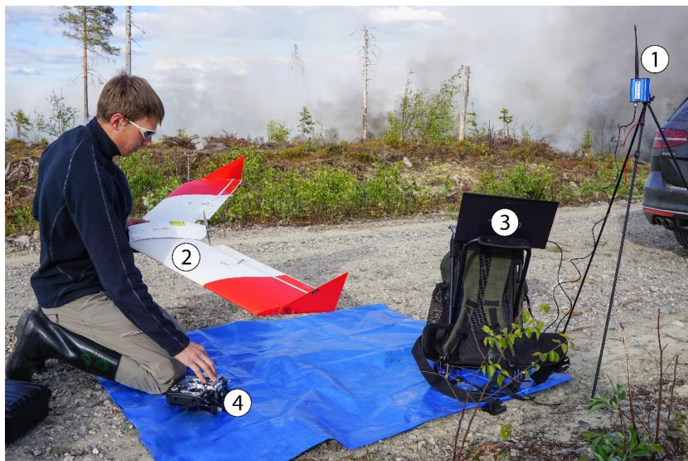
Figure 3.1 This is a typical setup when flying. The pilot performs a pre-flight check. Data Modem (1) communicates with the aircraft (2) in real time and via the ground station software in the computer (3) the pilot can obtain information on the plane's location, speed, incline, etc. The remote control (4) is used to control the plane during takeoff and landing, but at any time during the flight the autopilot can be used to manually control the aircraft.
