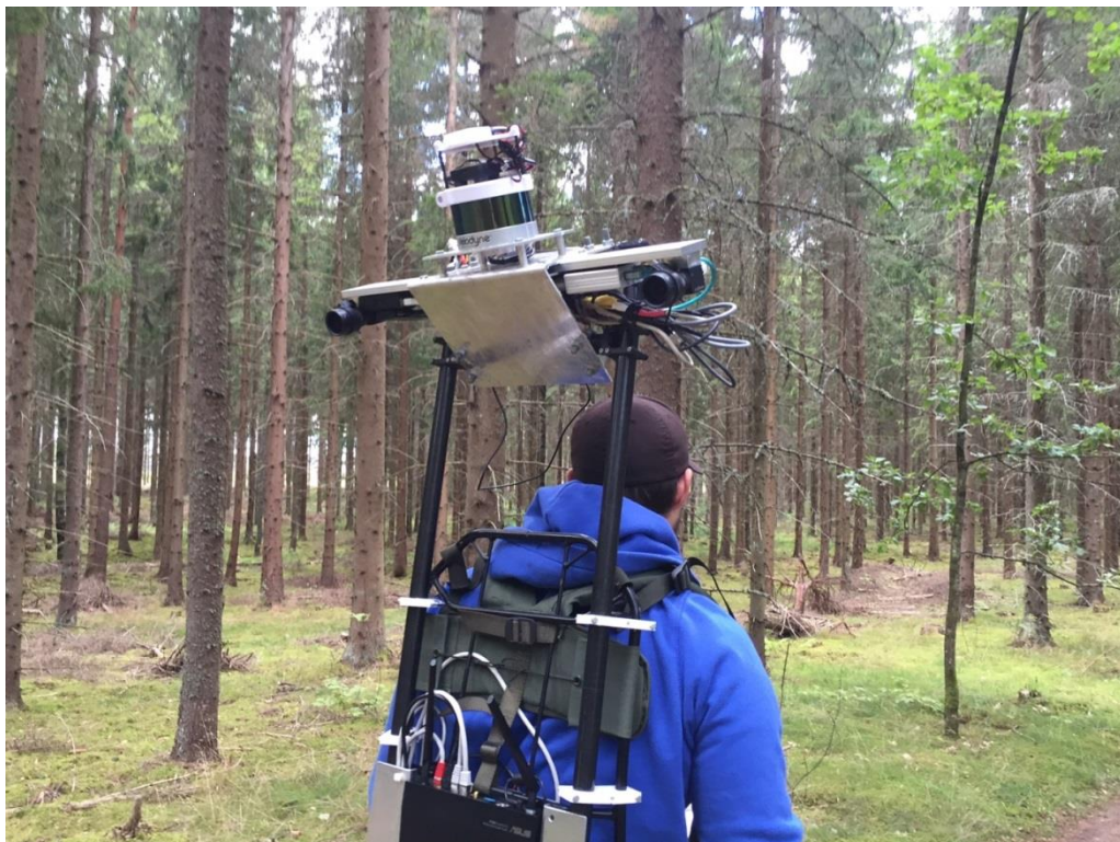
Figur 6.30. An experimental mobile laser scanning system with laser scanner, stereo camera, inertial navigation and computer for data logging and wireless communication network to other devices.
