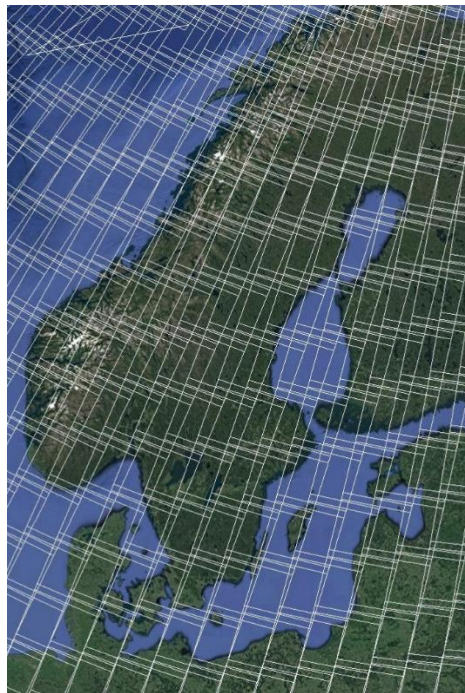
Fig 4.6 – The Landsat WRS-2 path and row system for identification of images. Image outlines are shown in white, and paths overlap.
